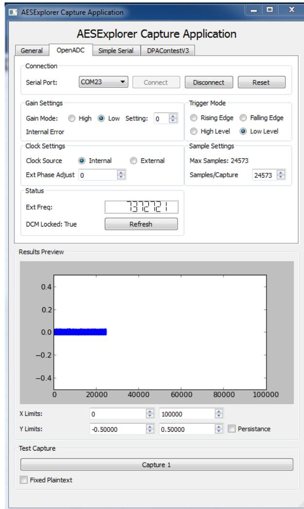
In the ‘Status’ field you can hit ‘Refresh’ and see if the external clock is working. You should see the correct frequency here should be around 7372800.
