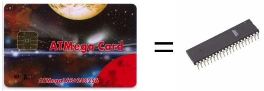
**There is no difference between demonstrating an attack on one of these Smart Cards and demonstrating an attack on a discrete AVR.** It's much easier to get a hold of discrete AVR's, so I don't even recommend bothering with the smart card attacks. Certain microcontrollers only come in the Smart Card form factor, so with those you **do** need to attack the smart card.
