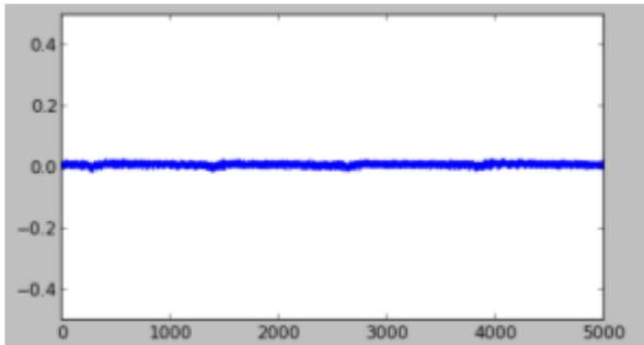
Finally we add a resistor in-line. This helps decouple us from the regulator to give us the final clean signal:
