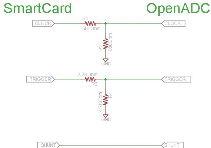
You MUST ensure the grounds of the two systems are connected for this to work! Note because the OpenADC as an AC-coupled analog input, the shunt line does not require any conditioning. Thus even though the shunt line is sitting at 5V, that will be fine.
