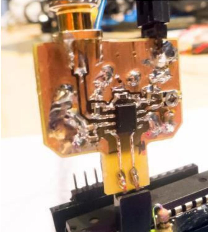
The critical part is the AD8129/AD8130 differential amplifier chip. You will typically add some gain right here, as that will reduce the ability of noise to affect the signal. How much gain to add is up to you – with the OpenADC you don't want too much gain, as the maximum input signal swing is limited.
