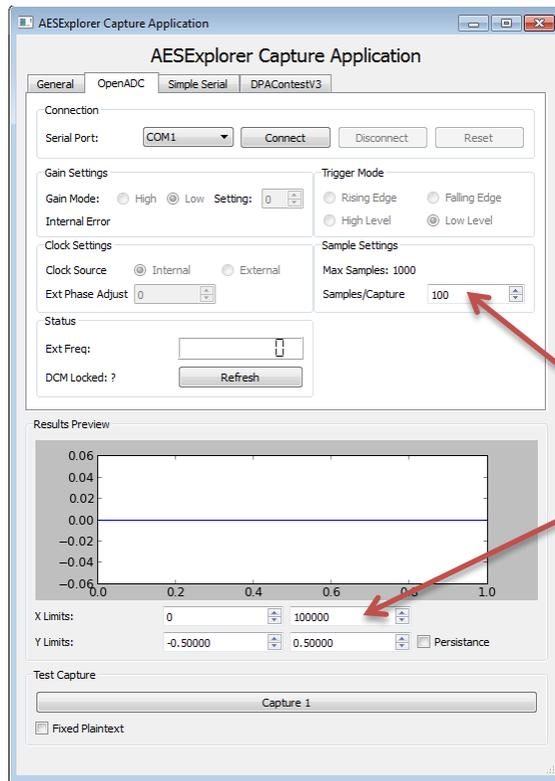
Select the proper COM port and hit 'Connect', assuming you are using the LX9 microboard with the OpenADC. You will probably want to adjust the 'Samples/Capture' and the 'X Limits' of the graph, those are highlighted in the previous image.
