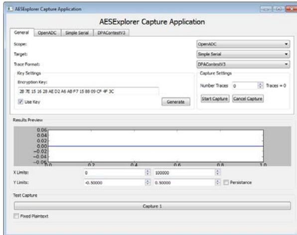
The ‘scope’ should be set to ‘OpenADC’. The ‘target’ should be set to ‘Simple Serial’, assuming you are using the targets described here. Finally you have the choice of how traces are stored – the default ‘DPAContestV3’ is a format defined for the DPA Contest V3 (see [dpacontest.org](http://dpacontest.org)). The DPAContestV3 is very straight-forward, and consists of text files with the saved waveforms & other required data.
