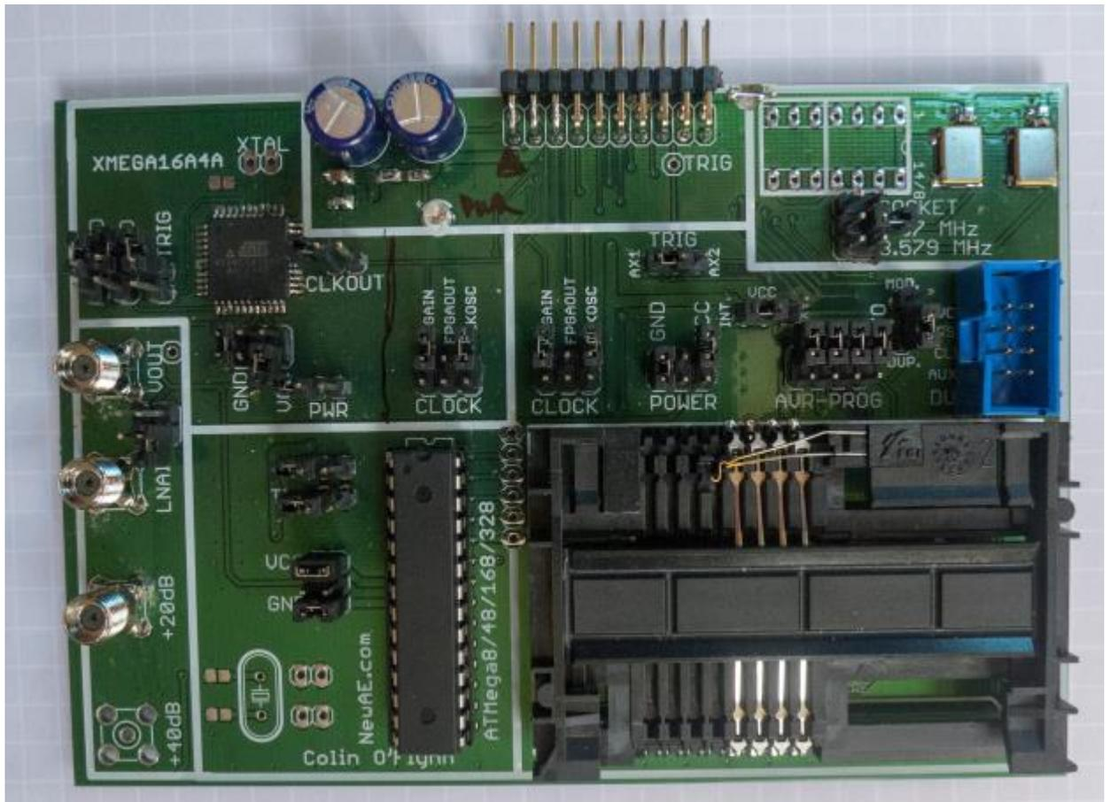
Note the board is specifically designed to work with the ChipWhisperer-Capture Rev2 Hardware. It can be used with other devices but will require some work breaking out the main connector.
