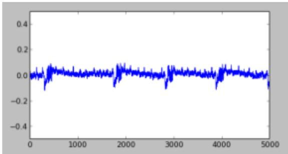
This is bad! There is far too much noise in this measurement! The voltage regulator for this example comes from a USB chip (CP2102), which has a fairly poor regulator! This is where all the noise comes from, so your systems will probably have less noise. Schematically, this looks like the following:
