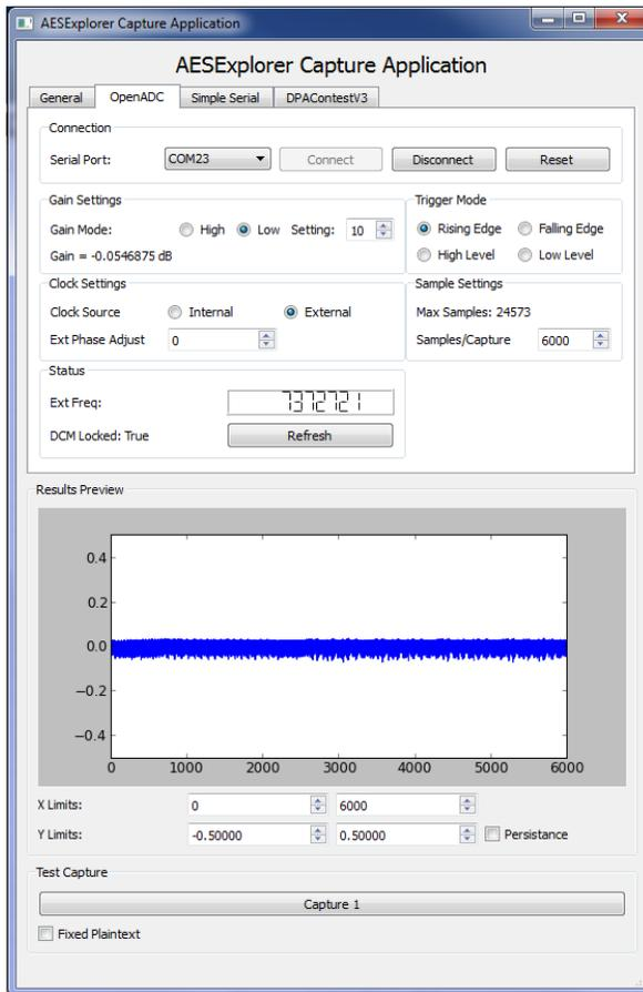
Ensure clock frequency is correct and 'DCM Locked' says 'True'.
