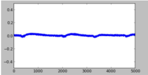
A slight improvement. Next we add a 680uF capacitor to try and even out the lumpy bits:
