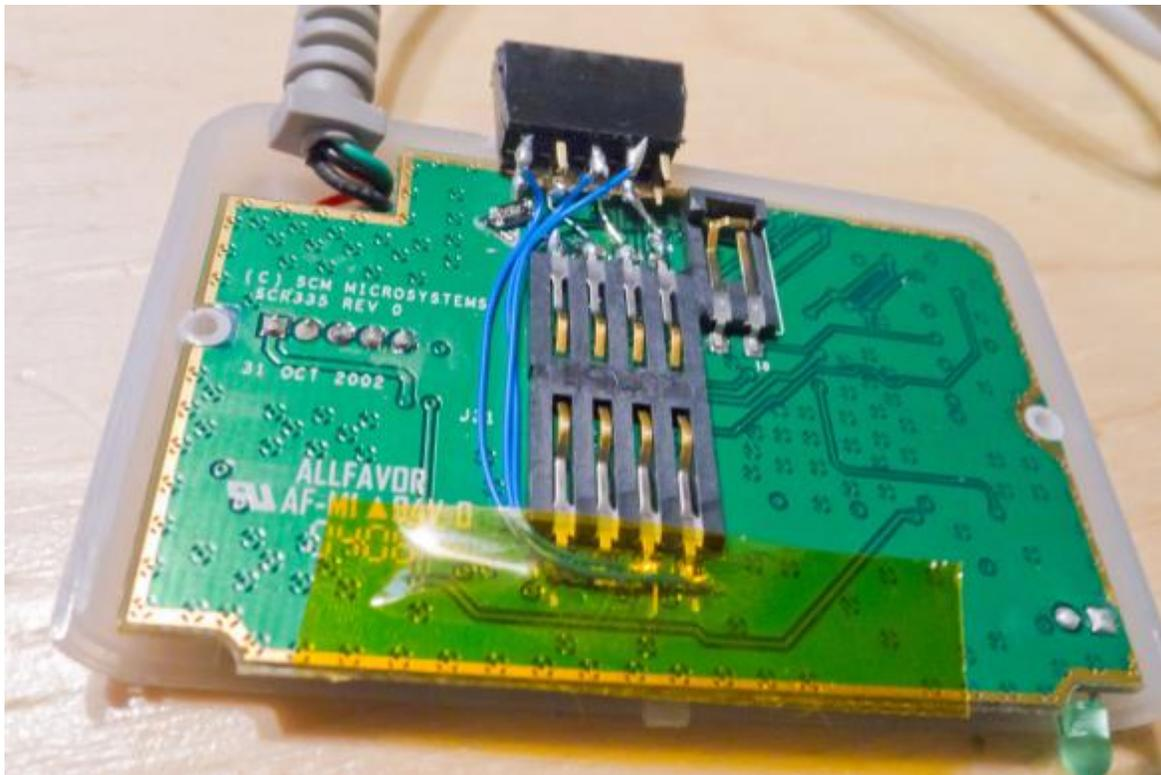
Close up the Smart Card reader, I added a connector on the backside:
