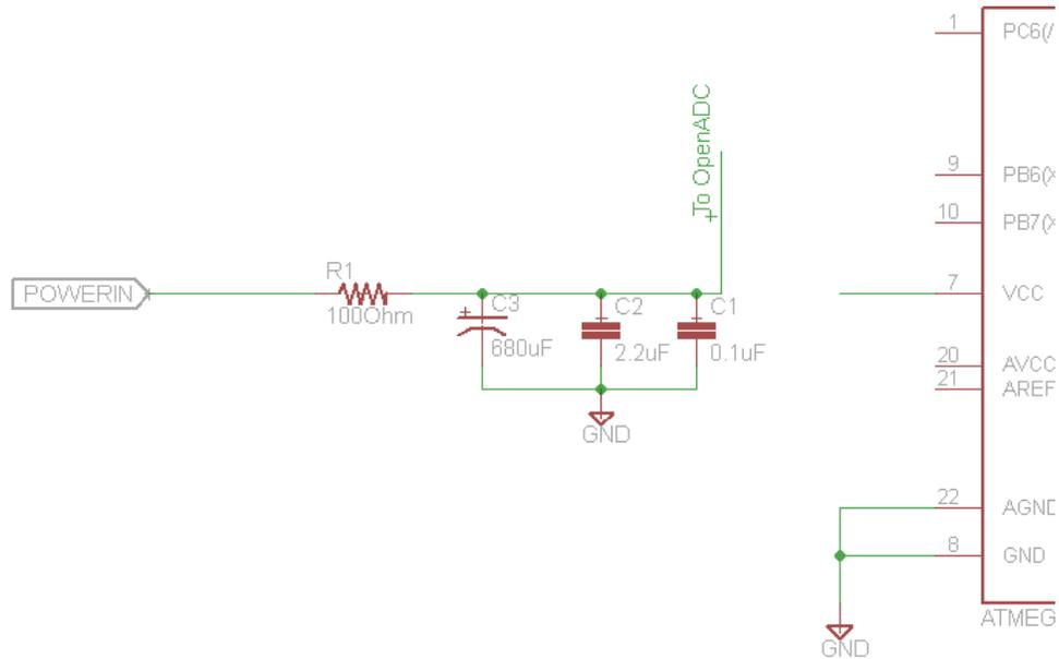
So to do the actual measurement we insert a shunt (and also connect up AVCC), and measure the voltage at the microcontroller side of the shunt:
