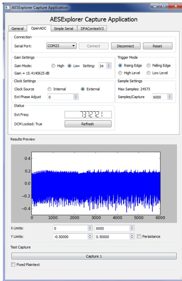
You can also adjust the ‘Phase Adjust’. This is highly dependent on your specific target. Some targets, such as the MEGA163 card, are very particular to the phase adjust.
