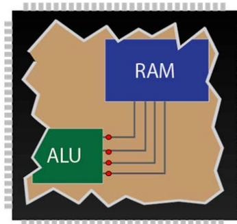
Well what happens when we send data across the bus? Power is transferred onto the bus from the VCC and GND lines. When we switch the states of the line it takes a charge – this means it takes power every time we want to change the state of the line.
