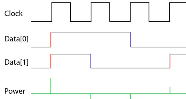
On each clock transition, it takes power to change the state of the line. If two lines change at once it takes more power than if one line changes at a time. What does this mean? We actually can learn something about the data on the bus.
