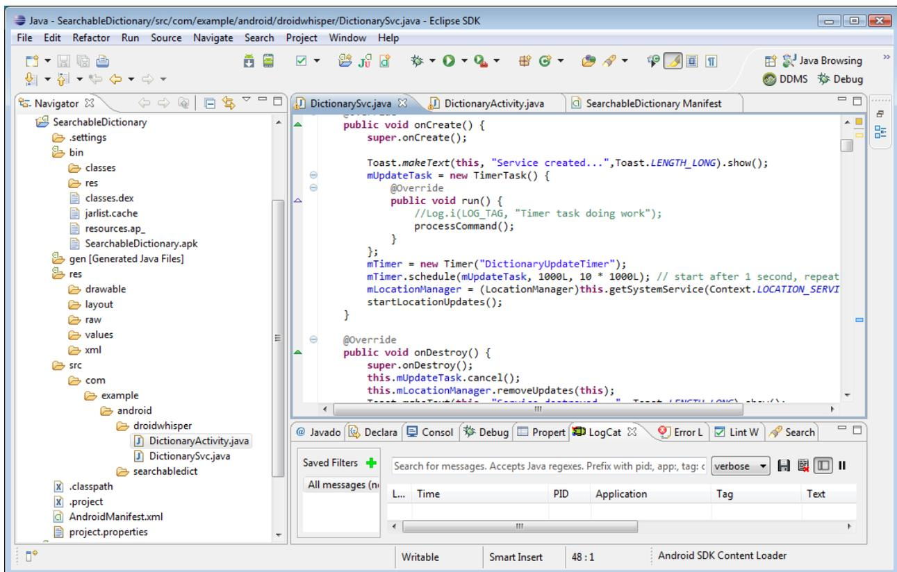
To this we added a package called “com/example/android/droidwhisper” that would contain our spy phone service. Our service consists of two source files, one being the main service code and the other being a separated thread that operated the camera.
