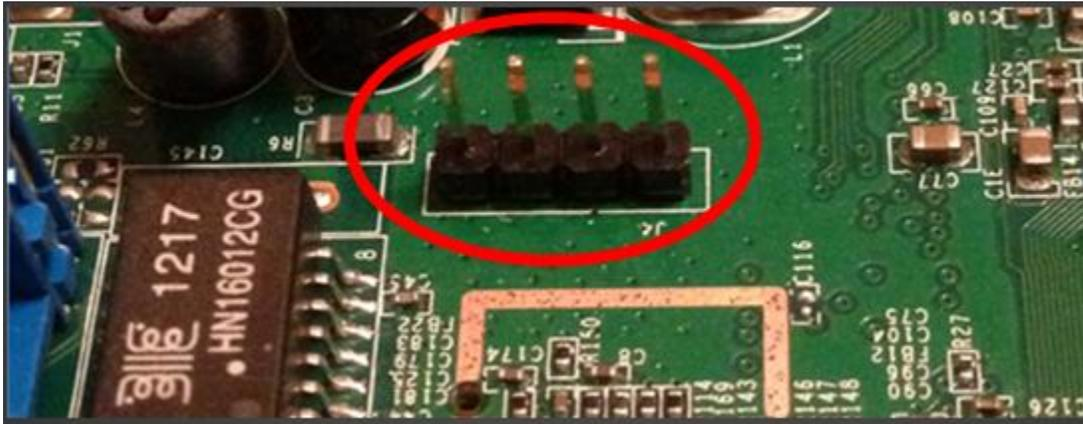
Figure 1 A common pin configuration for a UART interface
