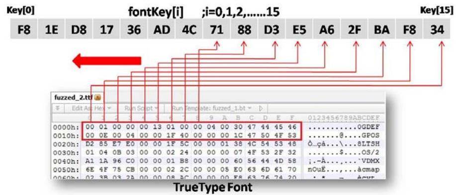
Figure 6: Performing the XOR operation on the first 32 byte of the TTF
